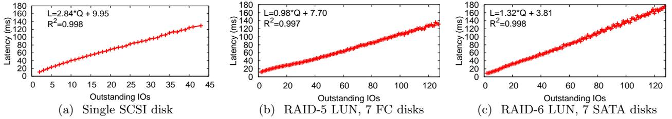
Figure 2: LQ-plots of latency *vs.* outstanding IOs show linear relationships for three different LUNs.
