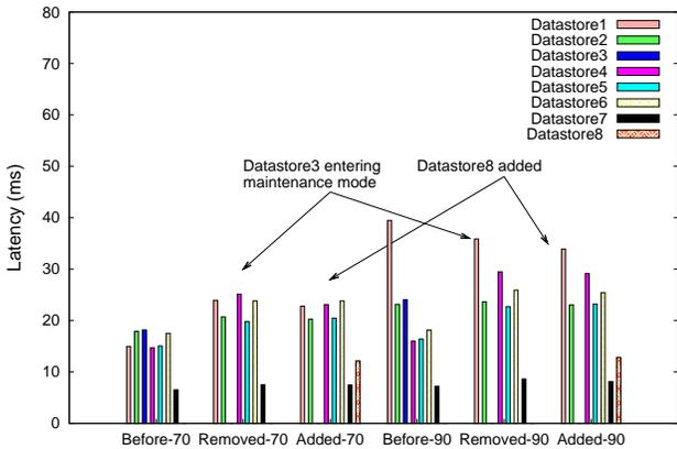
Figure 13: 70<sup>th</sup> and 90<sup>th</sup> percentile latency values before, after putting datastore in maintenance and adding a replacement datastore
