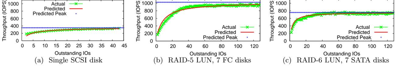
Figure 3: Plots of throughput (in IOPS) *vs.* outstanding IOs show non-linear relationships for three different LUNs. As the number of OIOs increases, the increase in throughput slows and ultimately saturates.
