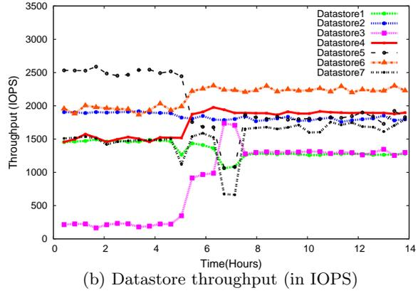
Figure 10: IO Load Balancing: Per-dastore latency and throughput observed during multi-hour experiment.
