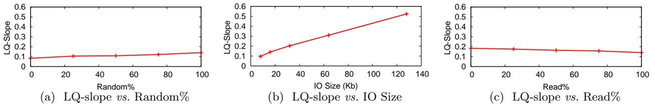
Figure 6: LQ-Slope as a function of IO workload parameters, for a 9-disk FC LUN.
