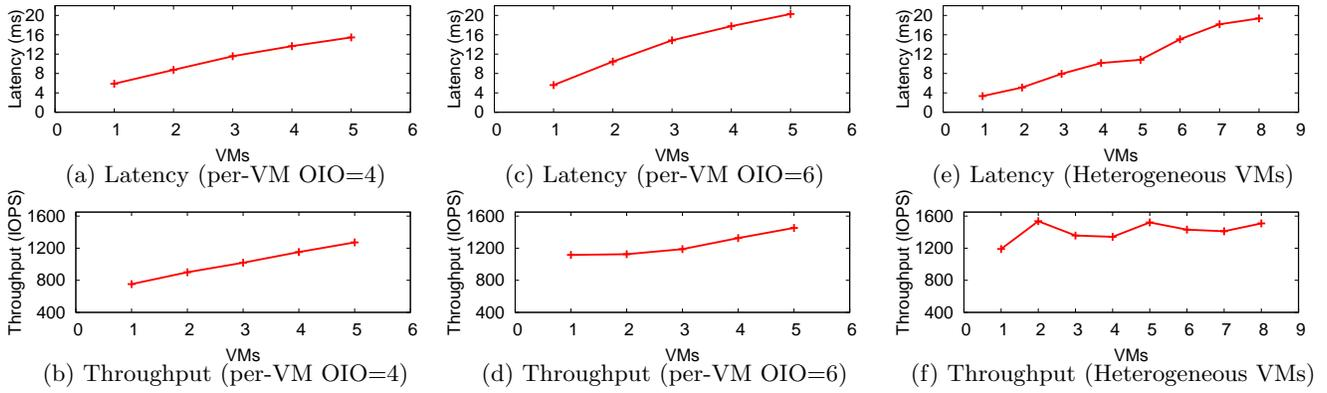
Figure 14: Capacity Planning: Predicting number of VMs to reach a certain latency or throughput value.
