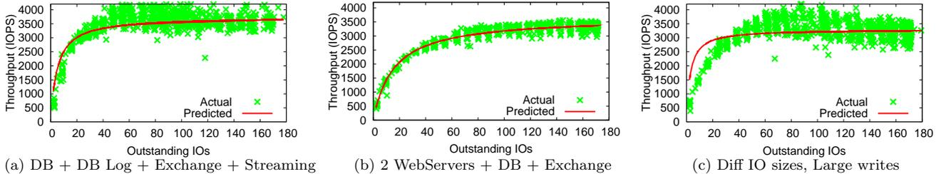
Figure 8: Throughput (in IOPS) vs. OIO relationship for three different workload mixes.
